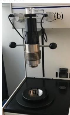
Figure 47. Photo de l'Autopore IV, (a) poste hautes pressions, (b) poste basses pressions
